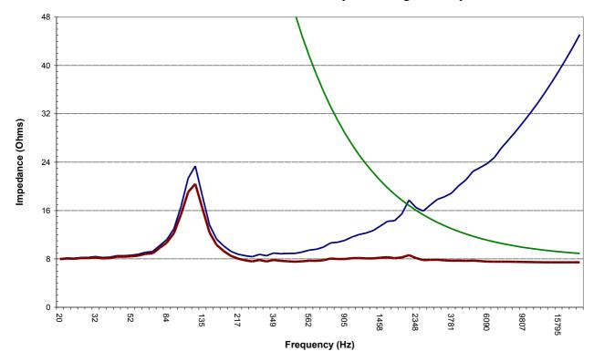
The Green line shows the impedance of the impedance correction circuit, the blue line is the impedance of the woofer and the red line is the result.
