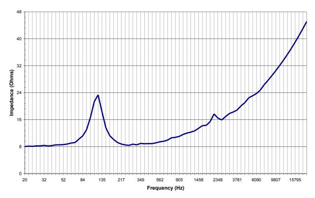
This speaker starts off near 8 ohms but by the time we get to 2.5Khz (a not unusual crossover frequency) the impedance has risen to 16 ohms.
