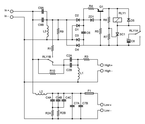
The circuit consists of three sections the Protection Circuit, the Low pass section for the woofer and the high pass section for the tweeter.
